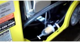
The lower hose connects the Fuel Filter Output end (right here) to a section of Fuel hose that connects to the Fuel 'T' connector that leads to the Fuel Pump and Fuel Selector switch. Note Fuel Filter has 2 clamps.
