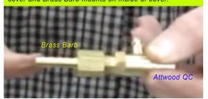
The Top hose connects the case mounted Brass Hose connector/Attwood Quick Connect. The off camera end is onto the barb of the Brass connect that is reachable on the inside of the Champion. The Fuel Filter end is connected to the Input side of the filter and secured with a clamp.
