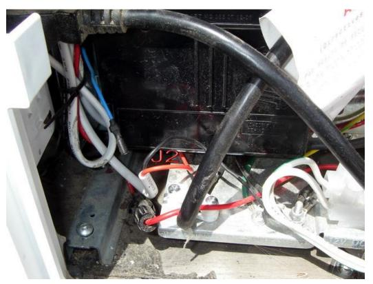
2. I then removed the light cover in the refrigerator and found the two red wires attached to the light switch. I pulled them out as far as I could and cut the one that was a larger diameter than the one identified in step 1.
