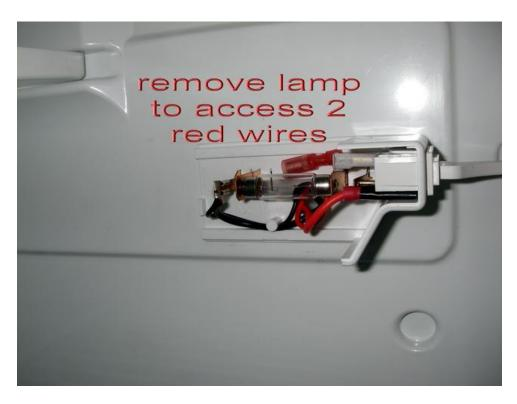
3. I then attached a female connector to the wire close to the switch and a male connector to the wire that goes through the hole in the refrigerator. I covered the male connector with electrical tape. If I need to use the heater in the future, I just join the two connectors.
