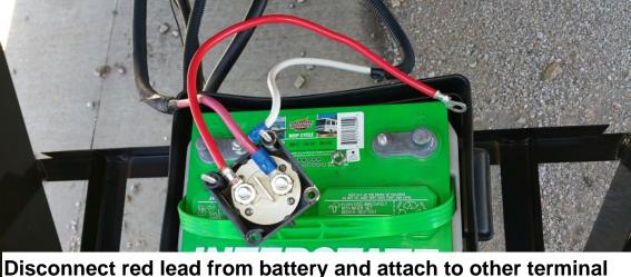
on switch. Had to drill out red connector to fit post on battery.
