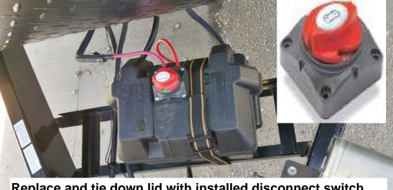
Replace and tie down lid with installed disconnect switch. Turn swith to red to disconnect battery - green to turn on.
