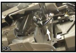
18. Insert a 1/2"-13 x 1-1/2" bolt and 1/2" lock washer, this hole may need to be reamed out slightly. Use one (1) of the 1/2"-13 nut plates to fasten securely.
