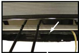
21. To install a breakaway switch, drill a hole to the side of the electrical rods. Be sure to place a piece of metal on top of the frame rail to prevent accidently drilling thru the radiator.
