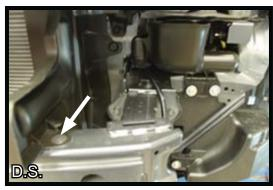
9. Using a flat screwdriver, remove the screw located on the top, outer edge of the bumper core. The bumper core will not get reinstalled.
