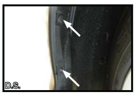
Using a Phillips screwdriver remove the screw at the bottom of the wheel well area. There are two (2) push pins that will need to be removed in this area also. Both are located above the screw.
