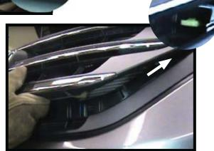
7. Look underneath the vehicle and toward the bumper to locate the four (4) yellow clips. Do this only to visually see where the clips are as you will be releasing them from the front side of vehicle. There are two (2) additional tabs on each side of the center of the bumper.
