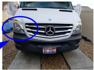
H7 Bulb is plugged into a mounting assembly. Replace mounting mounting assembly and bulb by accessing the rear of the headlight assembly from inside the motor compartment.
