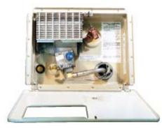
Another manufacturer, Suburban, uses a glass-lined steel tank in their brand of water heaters. The steel tanks require a "sacrificial" anode rod that attracts the corrosive elements in the water to itself, thus helping to extend the life of the water heater tank. This anode rod needs to replaced on a regular basis.
