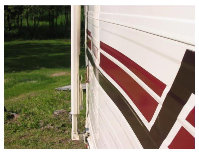
The above picture shows a bulge in the siding that indicates a delamination problem. The wall siding has separated from the Styrofoam insulation and a slight push on this area will show the extent of the damage. A bonded wall should be firm to the touch. The next picture shows the
