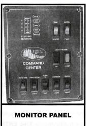
The monitor panel allows you to quickly check the levels in the fresh water and waste water tanks. Electrical sensors at various points on the tanks send signals to the monitor panel.
