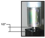
Pull the motor up until disengaged, about 1/2"
