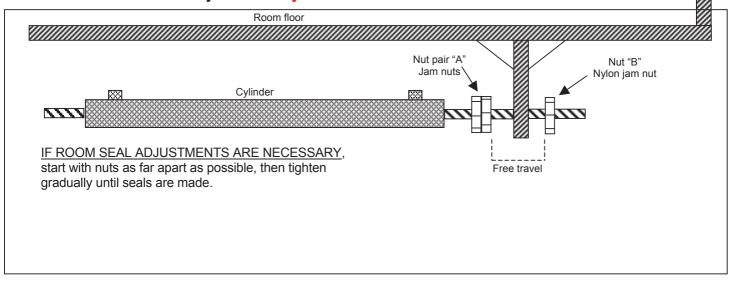
Jamb nuts are used to adjust tightness of room seals. Nut pair "A" in the OUT direction; nut "B" in the IN direction.
