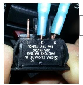
The existing switch that was in the convenience panel. It was being used as just an On/Off switch but can easily be made into an On/On switch.
