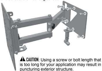
**STEP 3 Secure the television to mounting plate:** Line up the hole pattern on your television with the matching hole pattern on the universal mounting plate as close to the center as possible. Using the appropriate mounting hardware, washers, and optional spacers, secure the television to the mounting plate. This can be done without removing the mounting plate, figures are shown without bracket for illustration purposes only.
