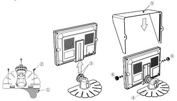
(1) Remove a protecting tape and attach stand place.
