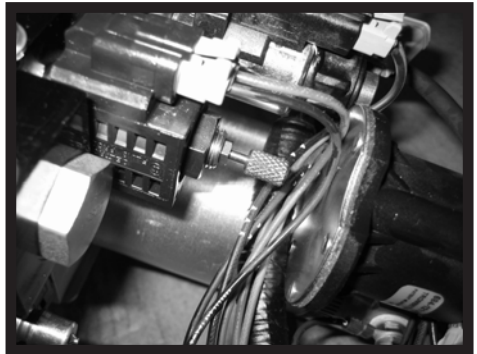
Release knob. Blue Knurled Knob should now be extended for manual override operation
