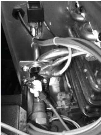
75C Limit Switch – White Switch 55C Limit Switch – Black Switch
