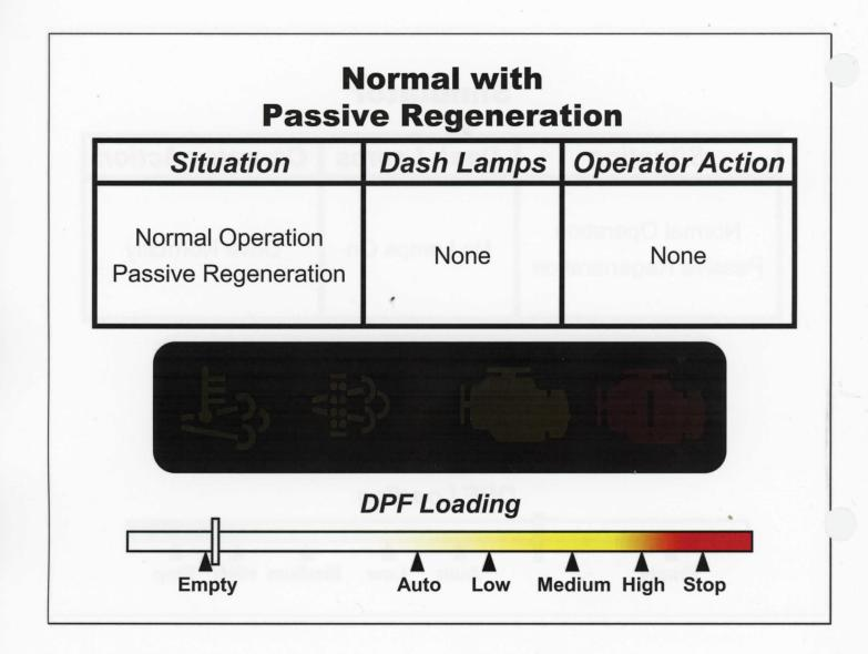
This slide relates to the normal operating mode or when the Aftertreatment system is in a Passive Regeneration mode.
