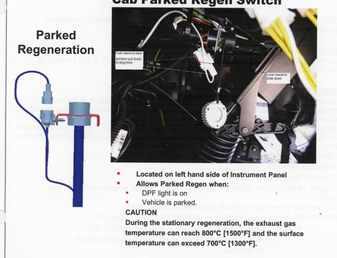
This picture shows where the new Freightliner cab switch for ISB07 CM2150
