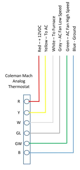
The thermostat is basically a switch that connects the red +12 VDC power to all of the other connections. If not battery powered, then a ground is required.
