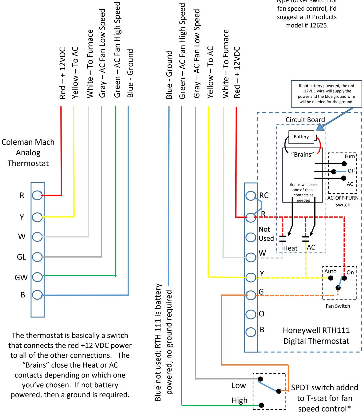
The thermostat is basically a switch that connects the red +12 VDC power to all of the other connections. The "Brains" close the Heat or AC contacts depending on which one you've chosen. If not battery powered, then a ground is required.
