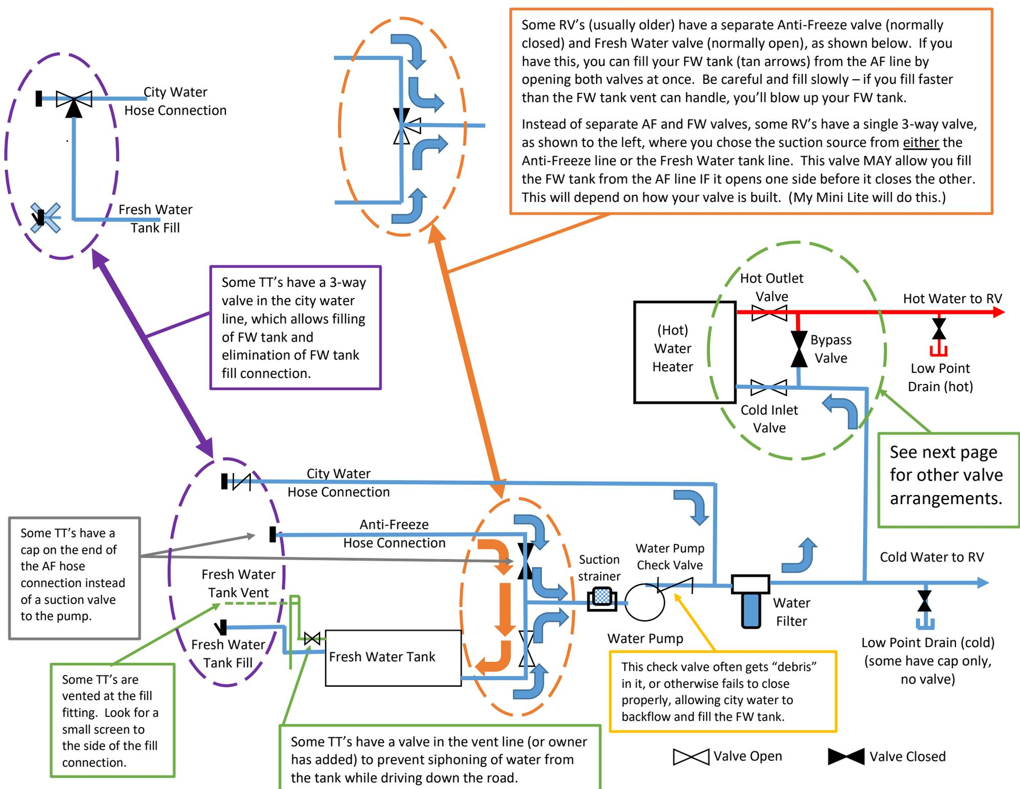
Some RV's (usually older) have a separate Anti-Freeze valve (normally closed) and Fresh Water valve (normally open), as shown below. If you have this, you can fill your FW tank (tan arrows) from the AF line by opening both valves at once. Be careful and fill slowly – if you fill faster than the FW tank vent can handle, you'll blow up your FW tank.
