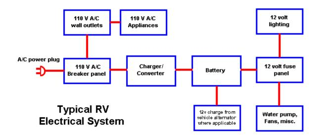
See.. there's really nothing to it! In the simplest terms, you have lights and other equipment such as water pump, fans, stereo, etc. that run on 12 volts, a battery that supplies the 12 volt power and some sort of charger to replenish the energy that you use from the battery. Of course, it's possible to add lots of useful components to this simple system to make it more flexible, but the basic 12 volt system in any RV starts with the components shown above.
