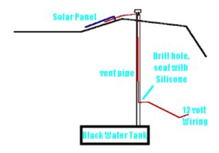
Once inside the RV, the wire can be routed to the location of the battery bank and connected to the charge controller.
