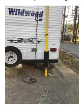
To the top of the pole I secure a pulley an run a 30 ft halyard to the ground to hoist up the center of the G5 RV. and raise it up. The pole is up in the top picture but extends beyond the photo.
