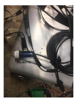
Pill Bottle sealed with hot glue joins Ladder line to Choke coax. Other end of choke is PL259 and Barrel connector.
