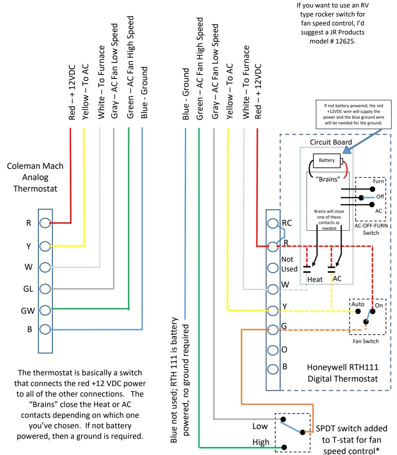
\*If you don't want to add the SPDT switch, just pick a speed wire and attach it to the G connection.
