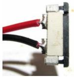
**Step #4:** Insert single color strip into connector opening, being careful to match the positive (+) and negative (-) marks on both strips. The bottom of the flex strip should be touching the black piece. Insert as far as possible.
