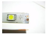
**Step #2:** If using our control cable, strip the casing approximately 3/4". Strip each small wire 1/8". For added protection, put a 1" long piece of heat shrink tubing over the wire (So that when you are finished you can position it over the connection).
