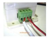
**Option:** You can connect more than one wire into each terminal on the terminal block. Simply follow the instructions above, making sure to pull on each individual wire when completed.
