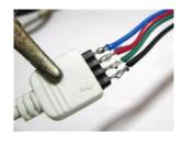
**Step #4:** Cover the connection with hot glue and/or heat shrink tubing.
