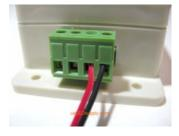
**Step #4:** Tighten down the screws above the wires you have inserted. Try pulling each wire out of terminal block in order to insure that they are fastened securely. If one is not secure, loosen the terminal and start over. Reinsert the wire and tighten the screw. The wires will be easier to insert if they are twisted first.
