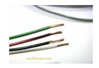
**Step #3:** With a hot, clean soldering iron, use Rosin-Core solder to pre-tin the solder pads and stripped wires with solder. It won't take long to heat the strip so be quick! You may double up the wires if you are going to be running several rolls or long distances.
