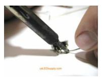
**Step #4:** Solder the pins to the LED strip. Then, cover your connection with hot glue and/or heat shrink tubing.
