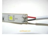
Step #4: Cover your connection with hot glue and shrink heat tubing.
