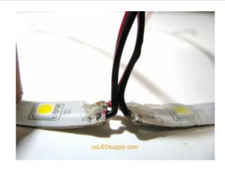
**Step #4:** Make a connection by inserting a pair of like-colored wires the entire way into the butt connector. With them inserted the whole way, crimp the butt connector with Channel-Lock or Robo-Grip type pliers.
