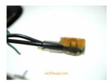
**Step #5:** Repeat the process (two wires per butt connector) for the remaining colored wire pair.
