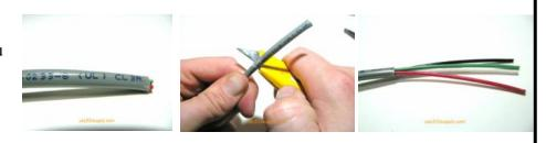
**Step #2:** Cut off the stripped ends of the wire on the flex strip. Peel apart the wires an inch back.
