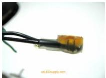
**Step #5:** Repeat the process (two wires per butt connector) for all of the remaining colored wire pairs.
