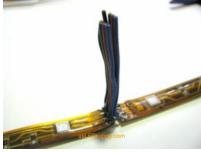
**Step #3:** Pull smaller wires apart. Then, twist same colors together.
