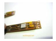
**Step #2:** Take a look at your 4 pin connector and compare it to the one pictured here. The pins on the right (with the thicker cylindrical base) will be the ones inserted into the IR controller, i.e. NOT the ones you will be soldering to the strip. You will be soldering the pins on the left hand side of this picture to the strip.
