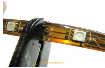
**Step #2:** Remove about a ¼" of the waterproof coating from the end of the strip. You may use your fingernail (if you use a knife be very careful not to cut through the circuit board). \*Note: you can leave the coating on if you will not be connecting to this end of the strip.\*
