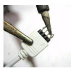
**Step #3:** Solder the 4 pins to the stripped wires, keeping the wires in the same order. It is helpful to use a clip to support your connections while soldering.
