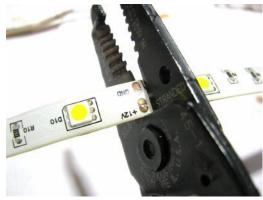
**Step #2:** Remove about a ¼" of the waterproof coating from the end of the strip (only if you will be connecting to this end of the strip). You may use your fingernail (if you use a knife be very careful not to cut through the circuit board).
