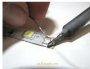
**Step #3:** Set the stripped wires of the male barrel plug onto the pre tinned solder pads, red for (+) and black for (-). Solder the wires to the solder pads on the LED strip.
