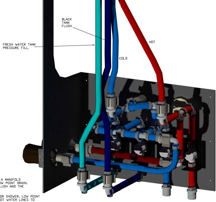
OFF OF CITY WATER INLET, MAKE A MANIFOLD TO CONNECT FRESH TANK FILL, LOW POINT DRAIN, EXTERIOR SHOWER, BLACK TANK FLUSH AND THE SUPPLY TO THE REST OF THE RV.
