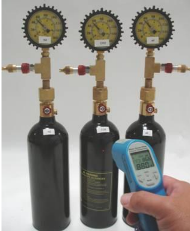
Figure 3 - Our shop temperature was 88°F so this became our next test temperature. All bottles were allowed to stabilize at this temperature for at least three hours. As you can see the pressure on the gauges of all of the bottles is virtually identical at 52 PSI. So far all of the gases have increased in temperature by 99°F and in pressure by 12 PSI.
