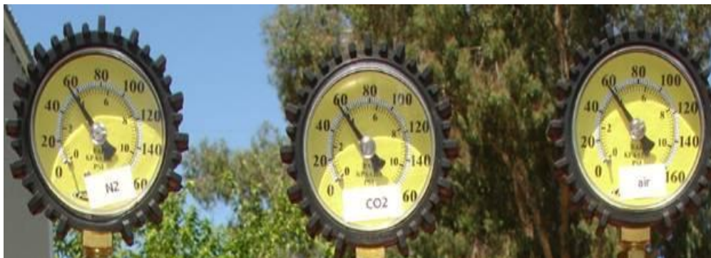
Figure 5 - At 117degrees F our gauges show a near identical pressure on all of them at ~57 PSI. Note: The "air" bottle gauge seems to show a higher pressure than the other gauges This is due partly to the angle of the camera to the gauge pointer. All gauges showed pressures within 1 PSI of each other.
