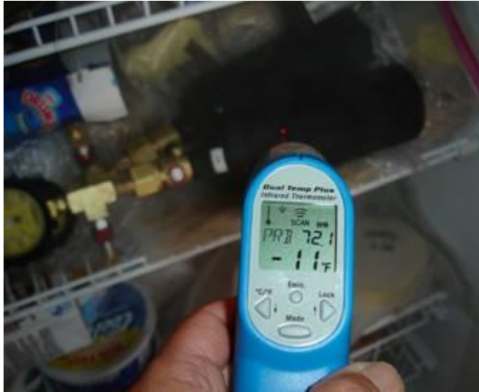
Figure 1 - I used an infra red surface thermometer to measure bottle temperatures. Each bottle was allowed to stabilize to temperature for at least three hours to ensure that the gas temperature was the same as the surface temperature. Our freezer got our bottles down to -11^{\circ}\text{F} in this test for a good starting temperature.
