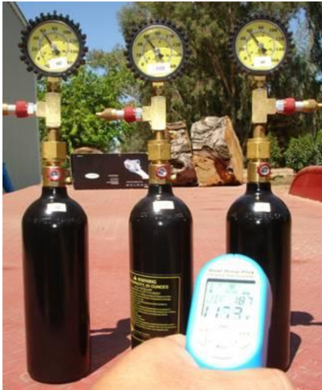
Figure 4 - We found out that if you stick a black aluminum bottle on top of a steel car hauler in the afternoon sun for a few hours you can get some damn hot bottles. You are seeing a bottle temperature of 117.3°F
