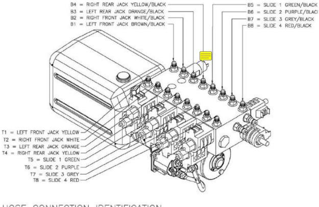
$\frac{\text{HOSE CONNECTION IDENTIFICATION}}{T = EXTEND}$ B = RETRACT
