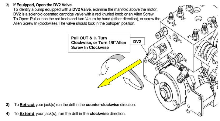
5) When Manual Override is complete, return the cartridge valve(s)
