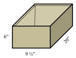
I used 1/2 "cabinet plywood for the drawer sides and 1/4" ply for the bottom. Once the drawer is built you mount the slides on the sides of the drawer. The drawer doesn't have to be exactly vertically centered in the opening as the front panel will cover any gaps between the drawer side and the opening.
