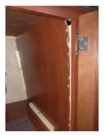
You'll see that this panel is held in place by some cleats along the back and bottom as well as being stapled along the front edge. The cleat screws are your standard #2 square drive type wood screws found throughout the camper. Remove the cleat screws and carefully pry loose the front edge. A cat's claw pry bar works well for this kind of work.
